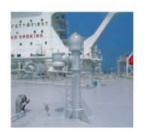
U-ISO-H/V/G series high velocity pressure/vacuum valve is designed to prevent the flame passage into cargo tanks and to relieve excessive over pressure or under vacuum of cargo tanks during cargo loading, discharging, ballasting and thermal variation.
